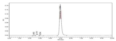
Figure.4c.Chromatogram of thermal degradation studies
