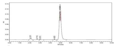
Figure.4d.Chromatogram of UV degradation studies
