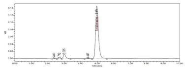
Figure.4b.Chromatogram of base degradation studies
