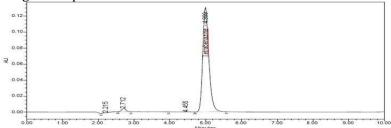
Figure.4a.Chromatogram of acid degradation studies
